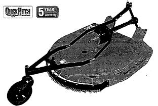
Hitch: 60" & 72" Cat. 1\* or 2 (QH Adaptable) 84": Cat. 2 Std. or Cat. 3 QH Adaptable or Pull-Type All Welded Deck Deck Height: 60" & 72" is 11<sup>1</sup>/4" 84" is 10<sup>1</sup>/s" Deck Thickness: 10 Gauge Side Panels: <sup>1</sup>/4"
